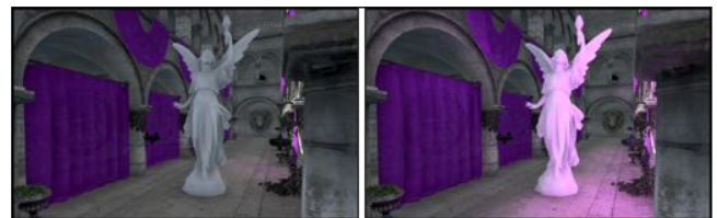
Figure 19: A single layer fails to capture indirect light from the purple banners behind the column in SPONZA (left), whereas our 2-layer Deep G-buffer captures enough light for plausible GI (right).
