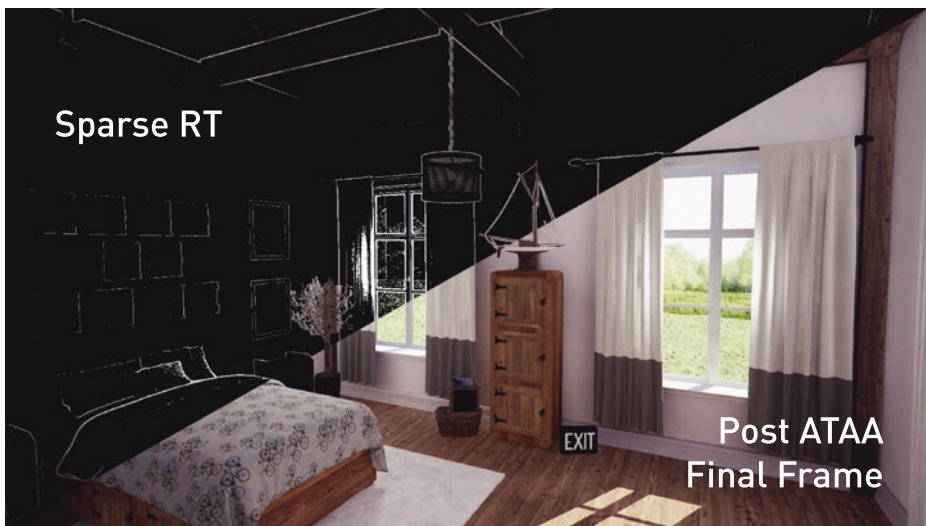
Figure 22-6. A cross section of an image rendered using our method, illustrating the result of the sparse ray tracing step (top) and the final composited ATAA result (bottom).
